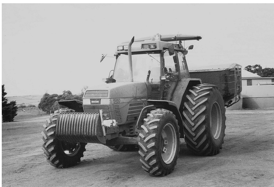
Figure 2. Yarra N Sensor on roof coupled to Bogballe VRT spreader and NTech GreenSeeker on front weights of tractor
