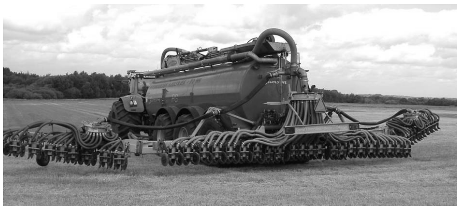
Figure 6. 14 m wide slurry injection system working on a controlled traffic layout
