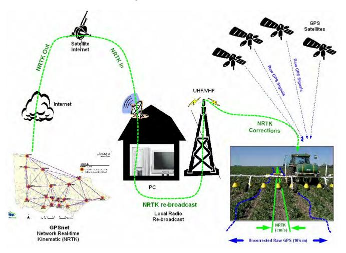
Figure 3. Schematic illustration of system data flow for the re-broadcast model
