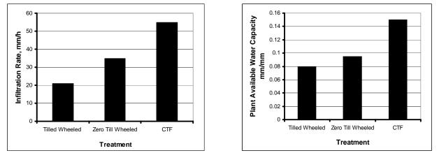
a) Infiltration rate during 80 mm/hour rainfall event b) Plant available water capacity (0 - 30 cm after two years CTF.)
