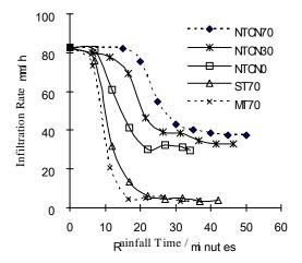
Figure 3. The change in inflitration rate with changes in level of compaction and cover. Where NTCN = No tillage no compaction plus cover (0, 30, or 70%), ST70 = compaction with small tractor (1.2t) + 70% cover, and MT70 = compaction with Medium tractor (3.6t) + 70% cover. (After Wang *et al.*, 2005)
