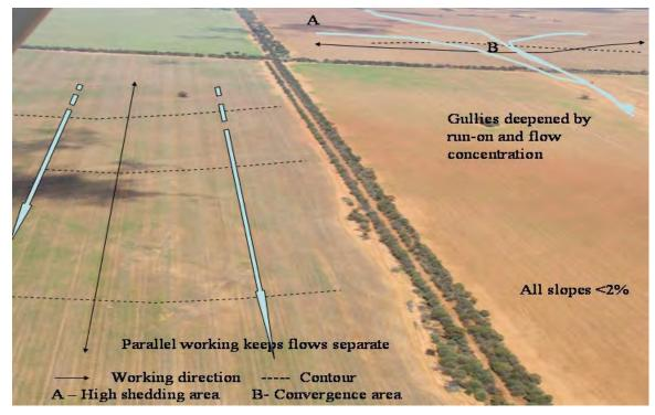
Figure 3- Aerial photograph (May 2005) of Sermon Road sites - contrasting effects of working up and down, and across the slope. Bottom left stable site in full cover and ungrazed; top right unstable site with low cover, run-on from high shedding area and flow concentrations by cross slope working.
