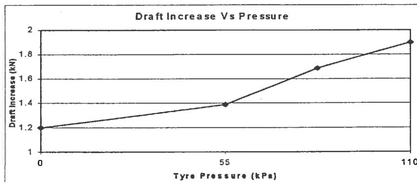
Figure 6. Draft Increase With Tyre Pressure – Trial F.
