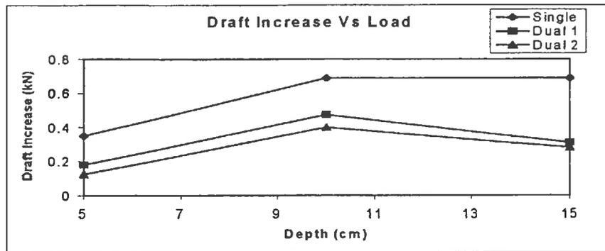
Figure 5. Draft Increase With Depth and Load – Trial F.
